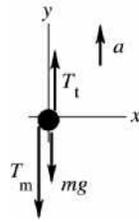
$$\begin{aligned} \sum F_y &= ma_y \\ T_t - T_m - mg &= ma \\ T_m &= T_t - m(g + a) = 120 \text{ N} - 2.00 \text{ kg}(9.80 \text{ m/s}^2 + 3.53 \text{ m/s}^2) = 93.3 \text{ N} \end{aligned}$$
